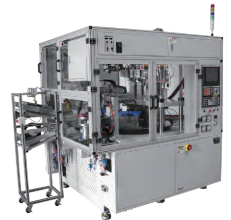
3 Injection & In-molding Assembly & Testing(Fully Auto)
