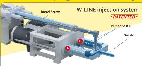
One extruder screw work with two injection plungers, the PET resin plasticizing, charging never stop by injection/holding process, compare to **In-line** screw, save 80% energy in charging.
